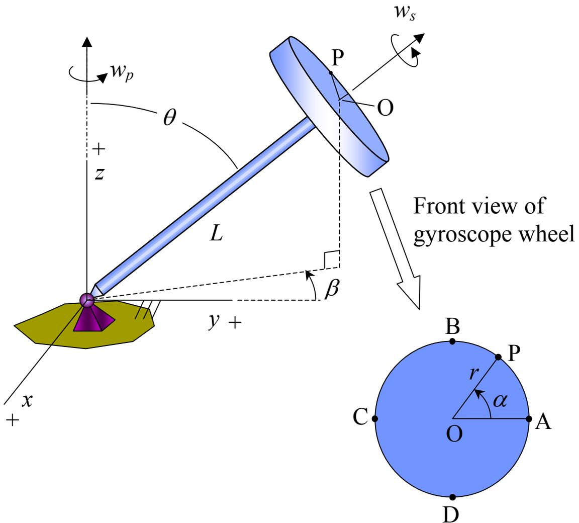
Define  $x_p, y_p, z_p$  as the coordinates of point P on the front face of the gyroscope wheel, relative to the reference frame  $xyz$ .
