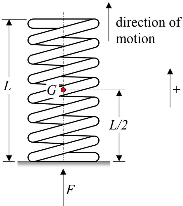
When the valve closes, the end of the spring (at distance  $L$ ) must remain in contact with the cam. Once the spring begins to lose contact with the cam we have a “valve float” condition, in which the spring is unable to “keep up” with the cam, and as a result is unable to match the engine speed.
