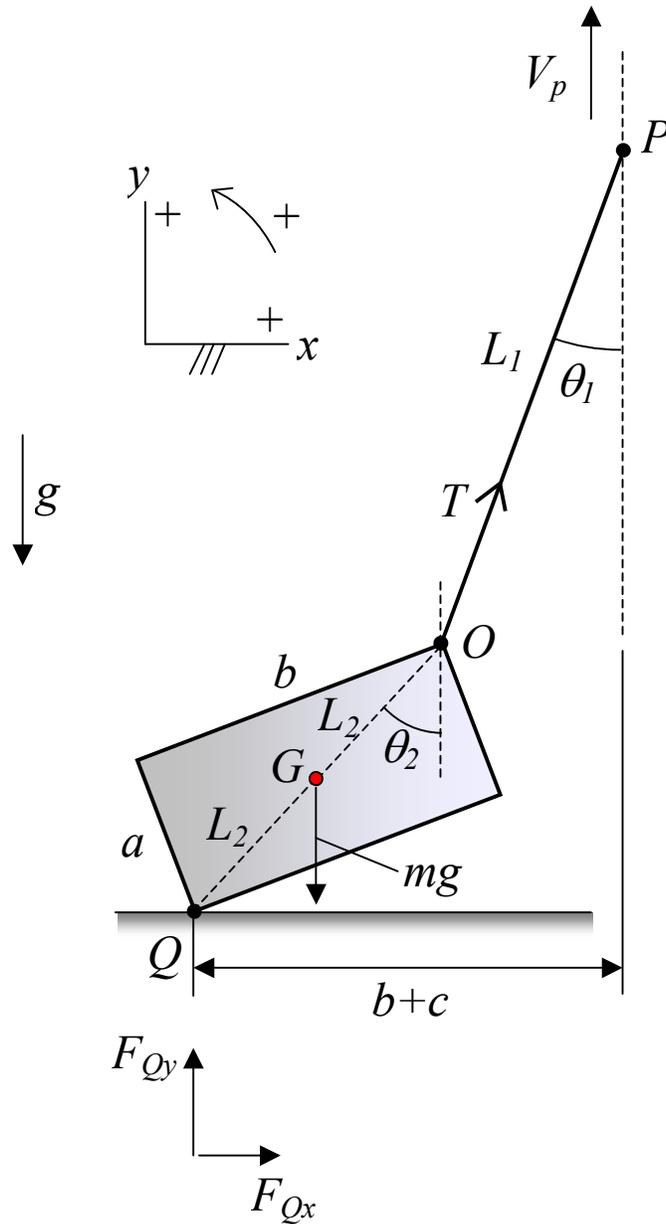
The pump casing lifts off when the vertical component of the cable tension  $T$  exceeds the weight  $mg$ . At this instant,  $F_{Qy} = 0$ .
