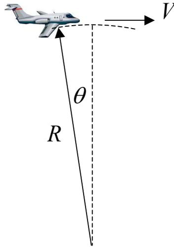
where  $V$  is the velocity of the airplane,  $R$  is the radius of the arc circular traveled, and  $\theta$  is the arc angle as shown.
