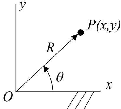
We wish to find a general equation for the acceleration of particle  $P$  along the radial  $R$ -direction. This equation can then be applied to the solution of this problem, which involves motion of the parts along the slots, which are aligned with the radial direction of the turntable.
