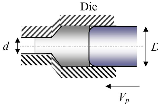
The force due to deformation of the aluminum during extrusion is given by
