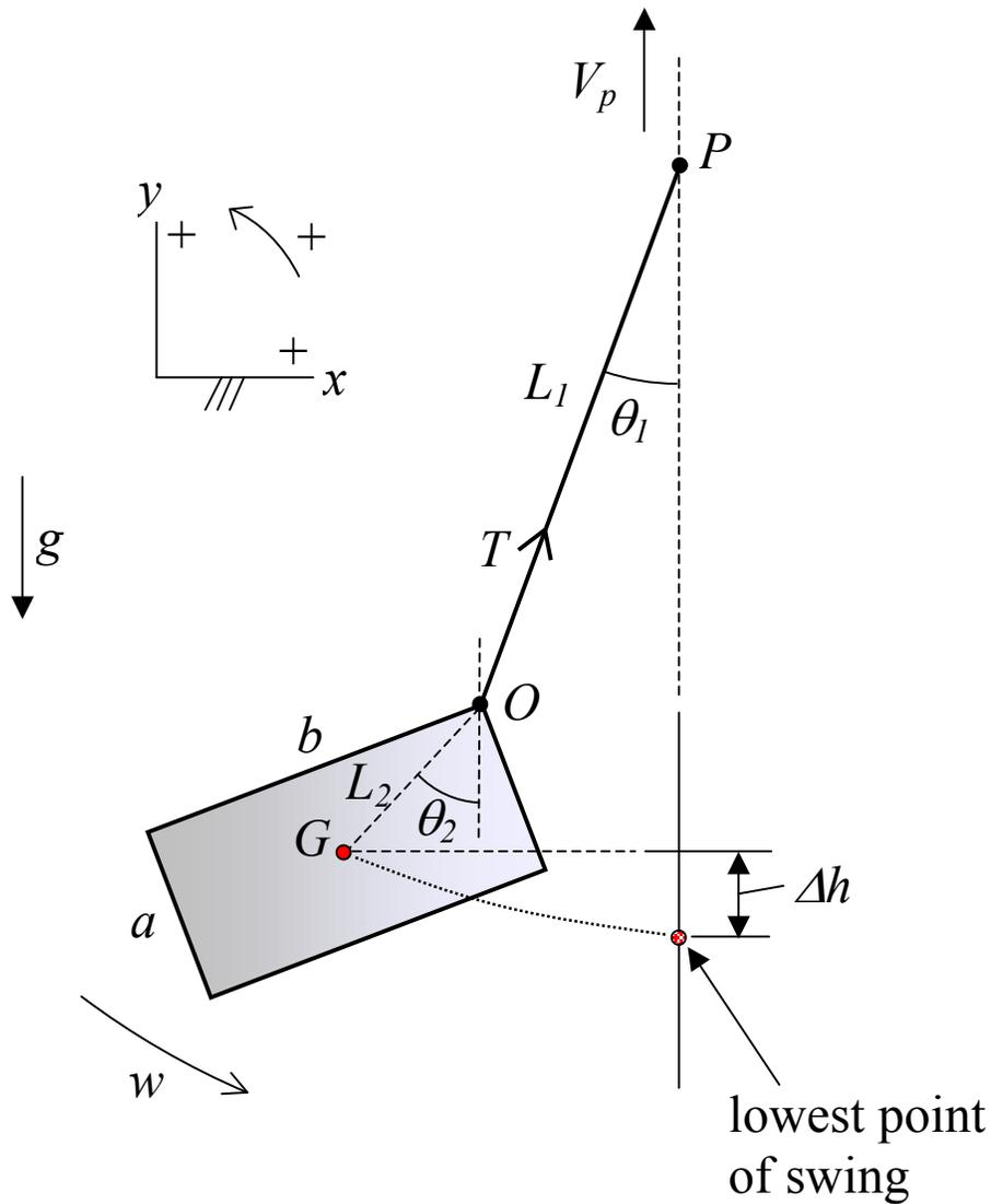
In the above figure, the variable  $w$  represents the angular velocity of the pump casing, and  $\Delta h$  represents the change in vertical height of the center of mass  $G$  of the casing, measured from the lowest point in the swing (the datum). At height  $\Delta h$  the angular velocity of the casing is zero since this is the highest point of the swing (and also where the swing starts).
