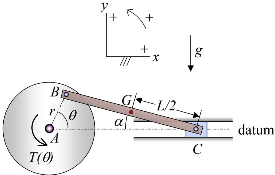
where point  $G$  (red dot) is the center of mass of the uniform linkage  $BC$ .
