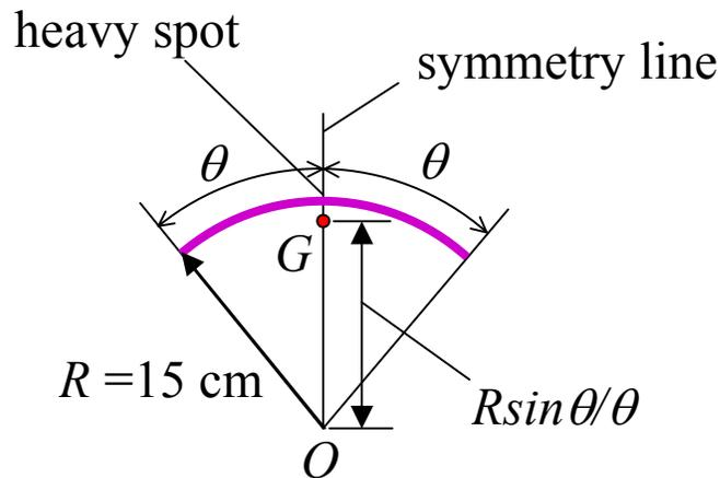
The point  $G$  represents the center of mass of the material removed from the groove. It is located at a distance  $R \sin \theta / \theta$  from the center of rotation  $O$  of the impeller (the angle  $\theta$  is in radians).
