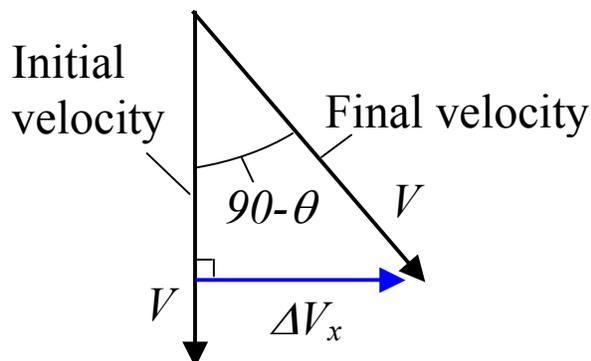
From geometry, the change in horizontal velocity of the material is given by
