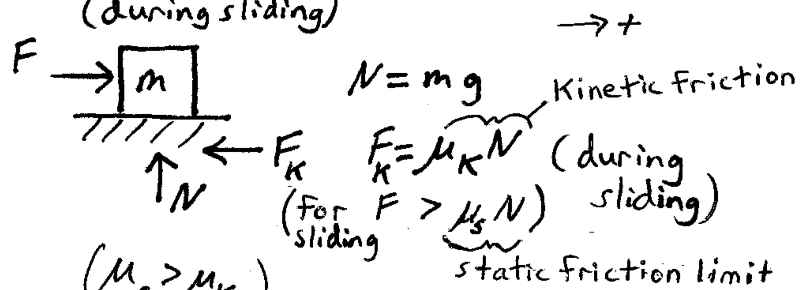
The block starts moving at time  $= t_0$ , when the static friction limit is exceeded.
