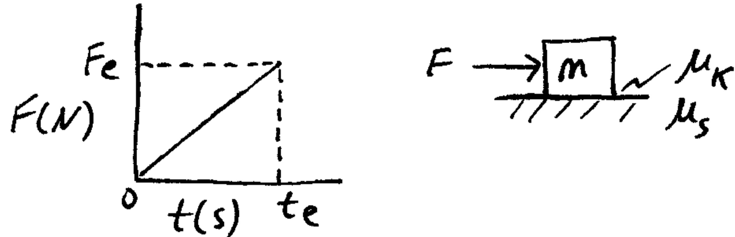
A block is initially at rest on a horizontal surface, and a force  $F$  is applied to it. Given the force vs. time graph, as shown, determine the velocity of the block at time  $t_e$ . Assume  $F_e > \mu_s mg$ .
