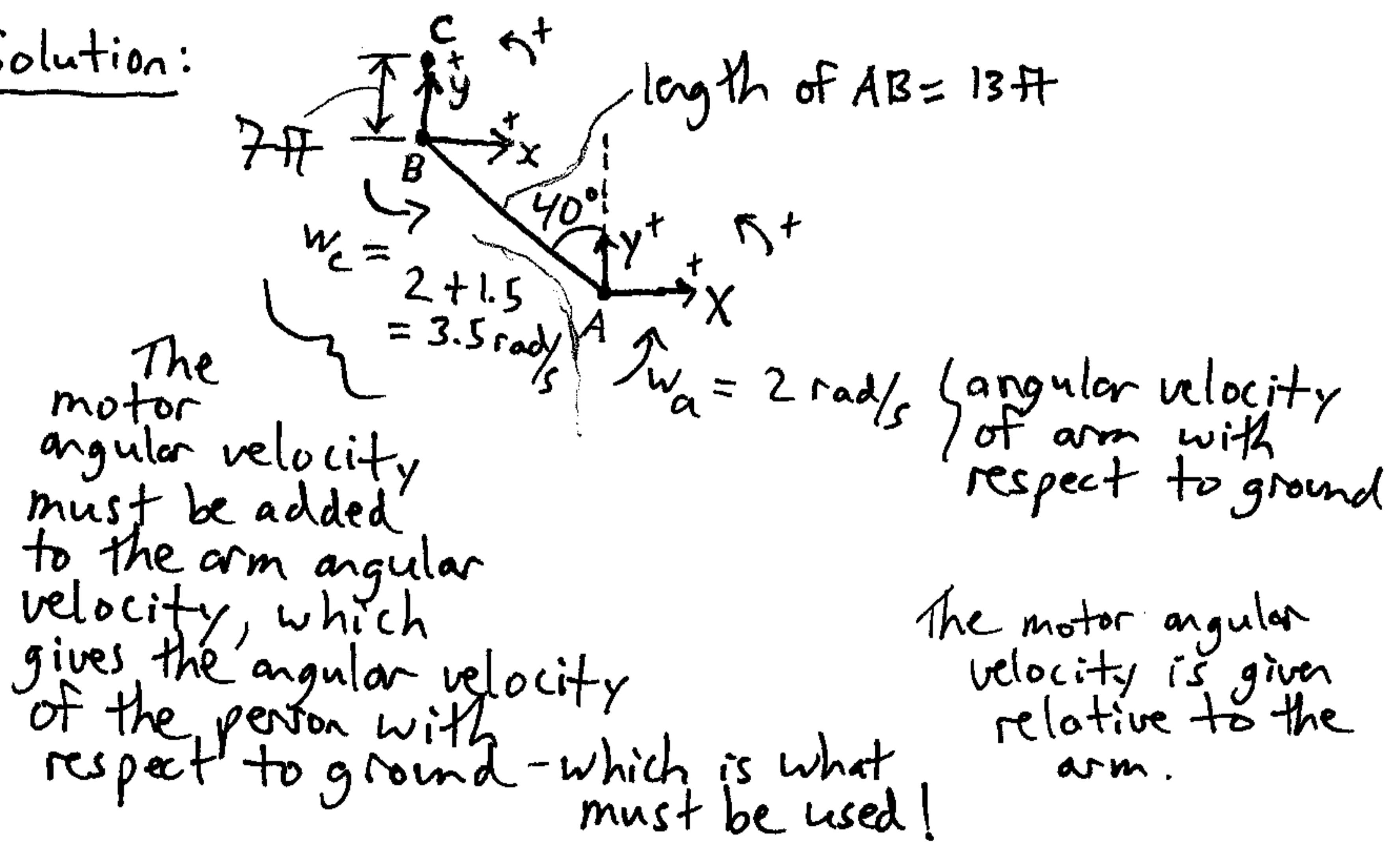
$$\vec{v}_c = \vec{v}_B + \vec{\omega}_c \times \vec{r}_{c/B} + (\vec{v}_{c/B})_{rel} \quad (I)$$
