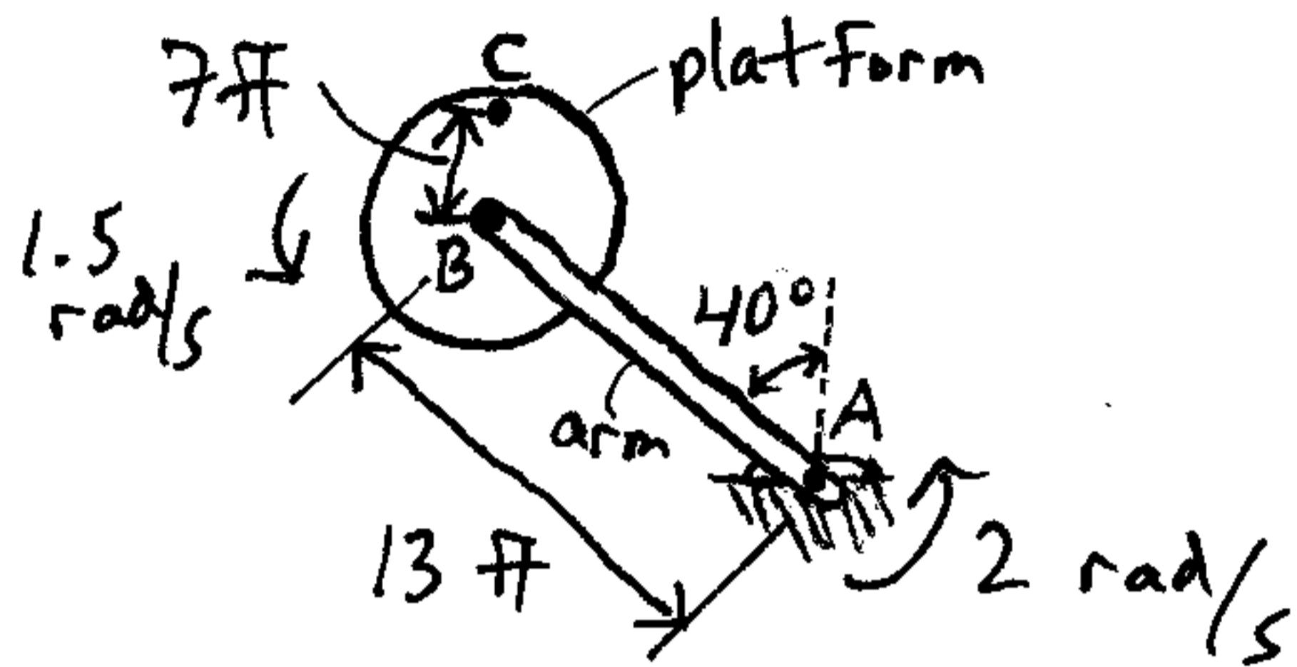
In an amusement park ride, the main arm is rotating about A at a constant angular velocity of  $\omega_a = 2 \text{ rad/s}$ . A platform is attached to the main arm and rotates about point B due to a motor which rotates at a constant rotational speed of  $1.5 \text{ rad/s}$ . A person is sitting on the platform at point C. At the instant shown, what is the velocity and acceleration of the person?
