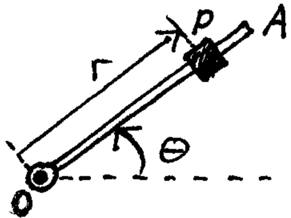
The rod OA is rotating in a horizontal plane about point O such that  $\theta = 2t^3$ , where t is in seconds. At the same time the collar P is sliding outward along the rod such that  $r = 40t^2$ . Determine the magnitude of the velocity and acceleration of the collar when  $t = 1.5\text{ s}$ . Distances
